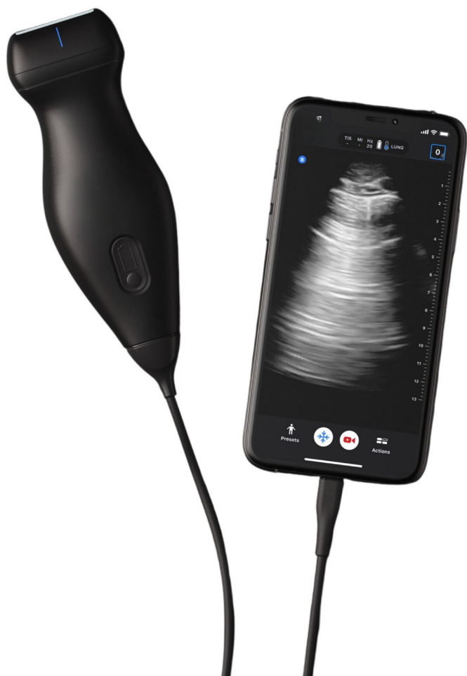
Figure 1 Portable one-probe point-of-care ultrasound device compatible with smartphone or tablet computer that was used during training and further practice.
